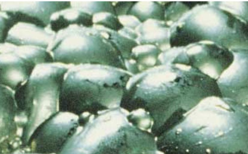
Molybdenite particles coat bubbles during flotation process
