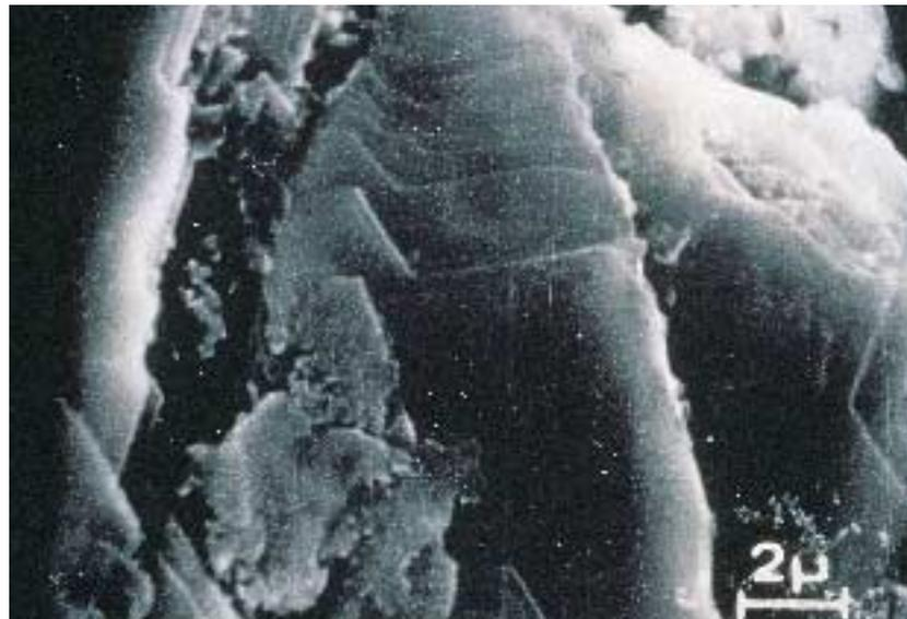
Cross-section of a molybdenum disulphide film showing the plate-like structure
