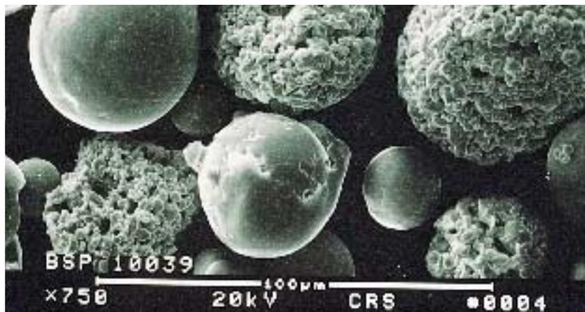
Spherical Agglomerates of Mo Powder (lacy appearance), with solid spheres of the Ni-Cr alloy binder for the Mo powder
