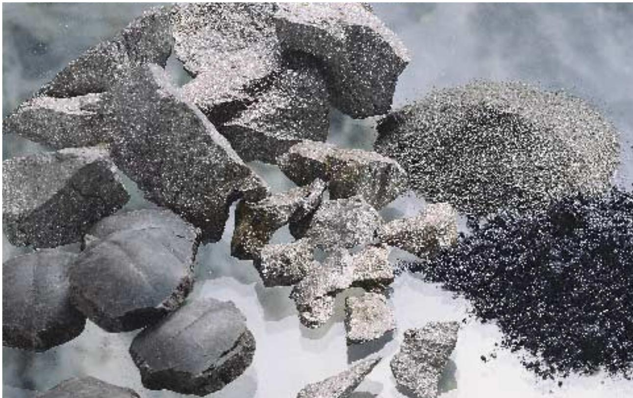
Samples of technical oxide and ferromolybdenum
